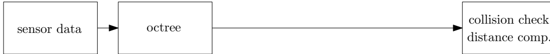
(b) By supporting the collision or distance query directly with the sensor data represented as an octree, we no longer need the long conversion pipeline from octree to broad-phase structures and thus can completely avoid the main overhead T_1 .
